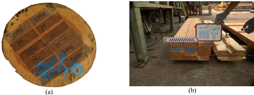
Fig. 2: (a) Manual positioning of the board end image for log #02 (flip means that the board end image had to be flipped to be in the right orientation); (b) A pile of boards from log #02.
